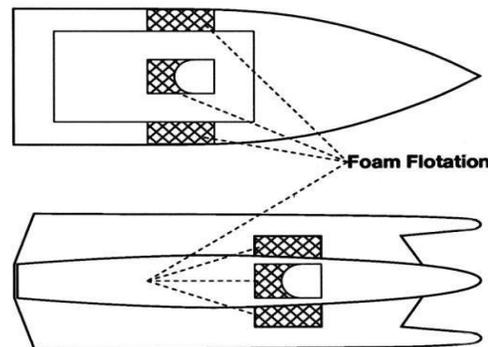
D. Boat manufacturers cannot count construction materials when calculating foam flotation requirements. Foam flotation will be added in the properly designated areas in the boat. (See Figure AA).
