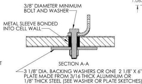
**NOTE: THIS SECTION IS TYPICAL OF ALL HARNESS ANCHORING TYPES THAT WOULD PENETRATE THE COCKPIT COMPOSITE STRUCTURE**
