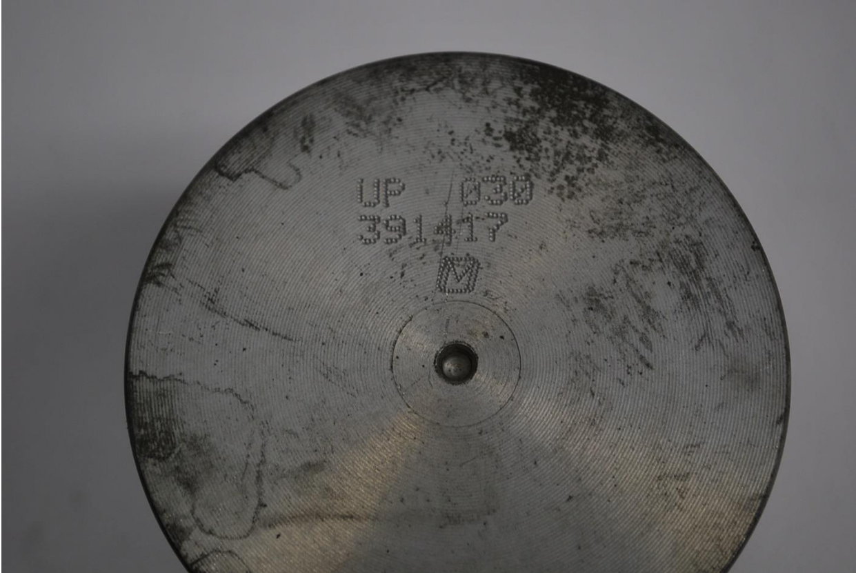
OEM Piston - PN 396581 – Distinctive OMC/BRP lettering on the top. No Boss on the wrist pin area of casting
